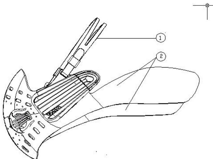
Hang 2 at the back of the neck and tighten up using Velcro so that both sides of the speakers stay close to the cheek bone near the ears. Wear 1 on the head and tighten the buckle above the ear.
